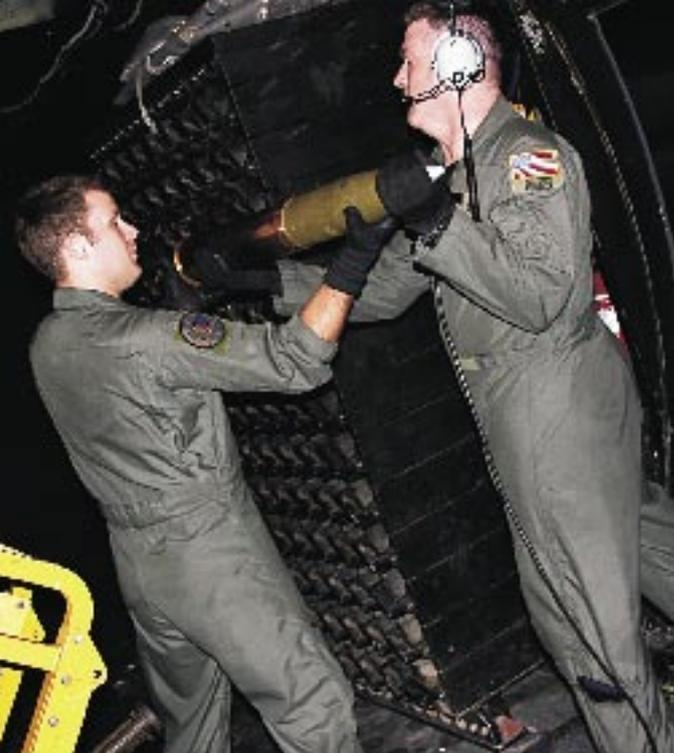
*Above, weapons loaders insert a 105 mm shell aboard the aircraft.*
